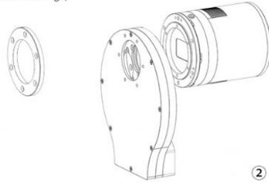
Note: Put OAG at the position next to M48/M54 Output to make both main cam and guiding cam focused.
