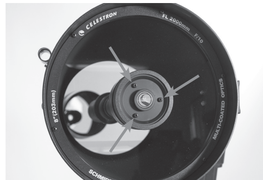
Secondary Mirror Collimation Adjustment Screws
