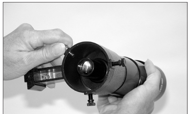
Figure 3b. Pull back the spring tensioning pin and slide the finder scope into its bracket until the O-ring is seated in the bracket ring.
