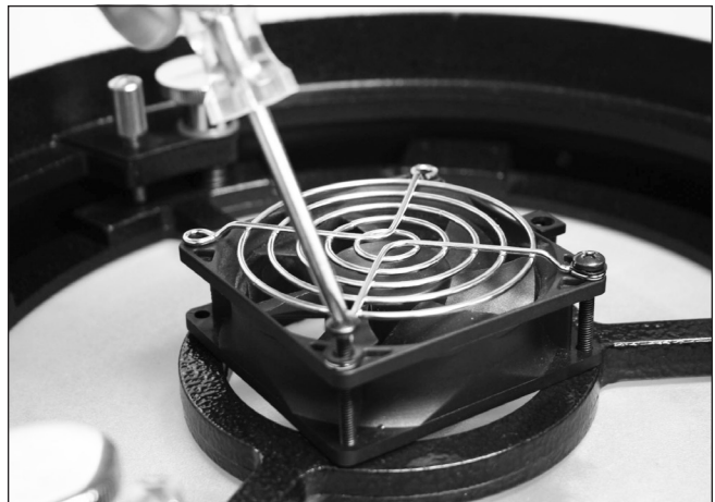
Figure 4b. Attaching the fan to the mirror cell.
