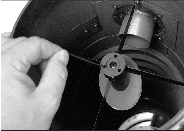
Figure 13. The tilt of the secondary mirror is adjusted with a 2mm Allen wrench on the three setscrews surrounding the center Phillips-head bolt.
