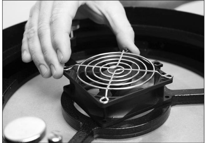
Figure 4a. Line-up the holes in the fan and fan cover with the holes in the rear of the primary mirror cell.
